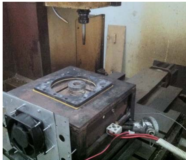
Fig. 5 Feedback thermal system is assembled to the SPIF feature
