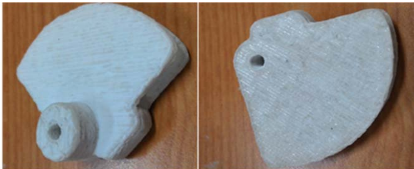
Fig. 11 Machine detail is made by SLS machine
