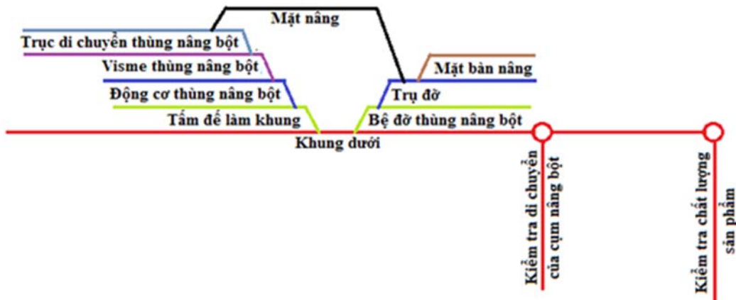
Fig. 7 Schematic diagram of the powder container installation
