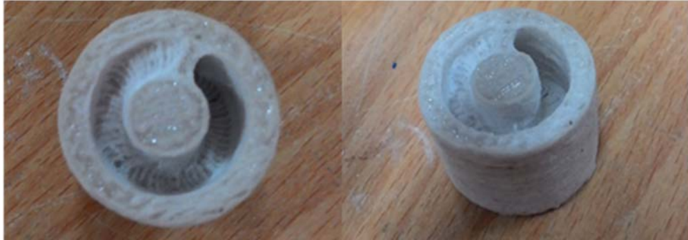
Fig. 12 Machine detail is made by SLS machine
