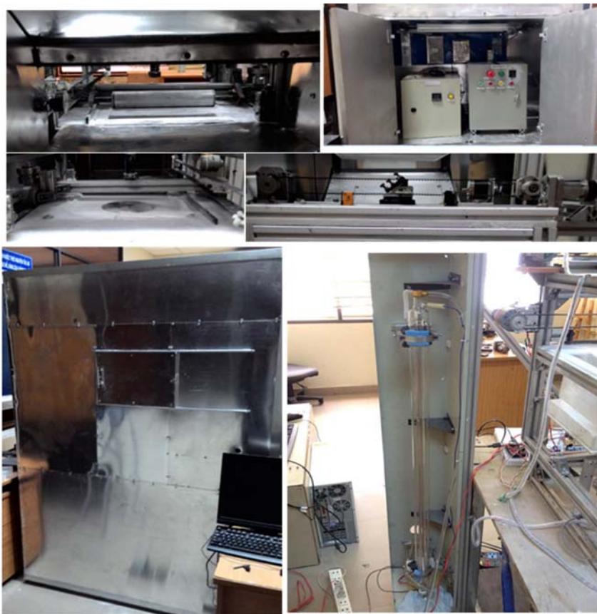
Fig. 3 The SLS rapid prototyping machine is completely manufacturing
