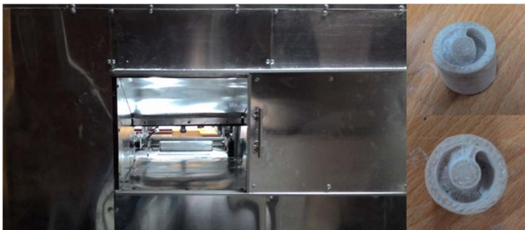
Fig. 11 Experiment and manufacturing products with SLS rapid prototyping machine.
