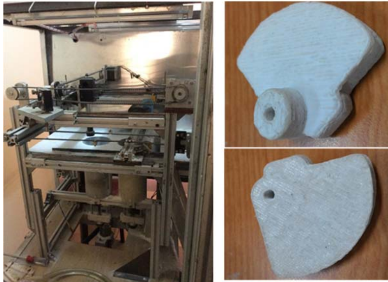
Fig. 3 SLS rapid prototyping machine and real products
