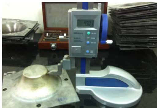
Fig. 10 Measure the bottom of the model after released from the feature to define the depth at breakage for deducing the angle \alpha
