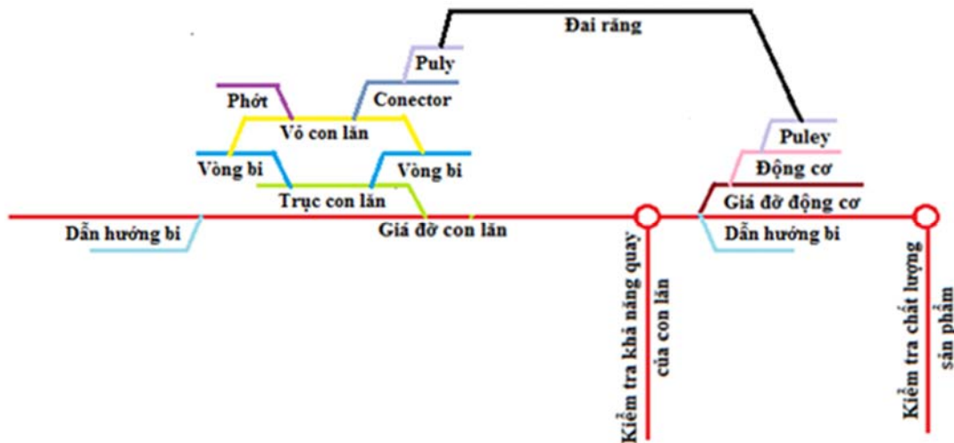
Fig. 3 Schematic diagram of powders roller installation
