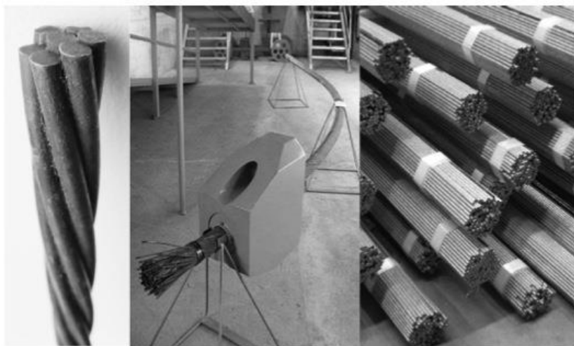
Figure 1.14 (a) High-strength nongalvanized 7-wire steel rope. (b) Helical strand, Little Belt Bridge. (c) Prefabricated parallel 127-wire strands.
