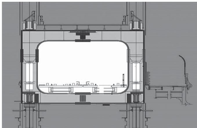
*Figure 1.9* Rigid frame constraining the end of each torque tube.
