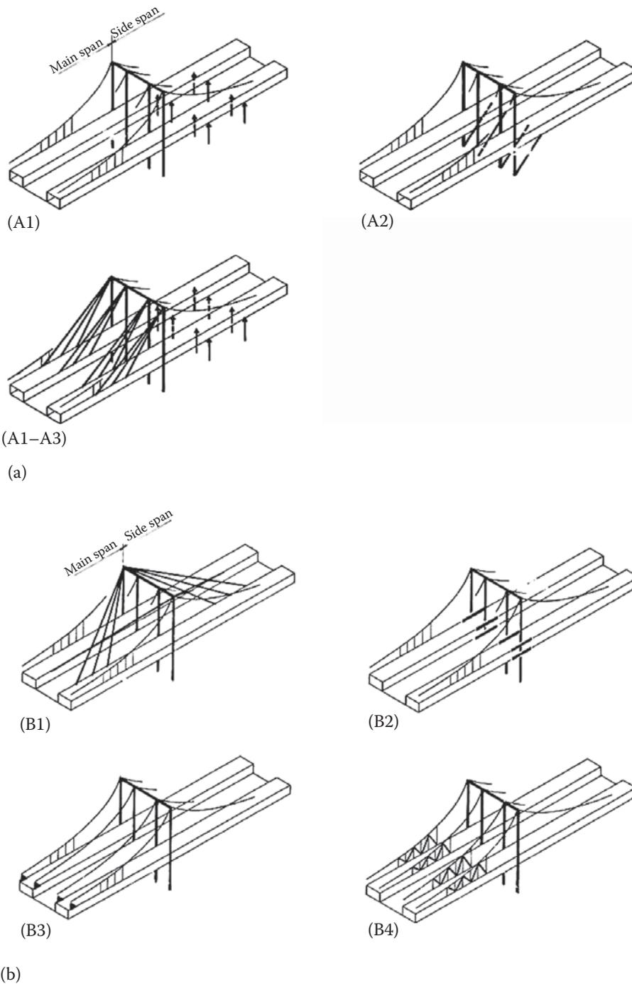
Figure 1.8 Stiffening schemes. (a) Category A: schemes that stiffen the category load; (A1) side span supports, (A2) underdeck cables in side spans, and (A1–A3) side span supports and stay cables in main span. (b) Category B: schemes that selectively stiffen the category load; (B1) crossed stay cables, (B2) interconnected hydraulic cylinders in truss chords, (B3) center span cable to truss connections, and (B4) diagonals between trusses and cables.
