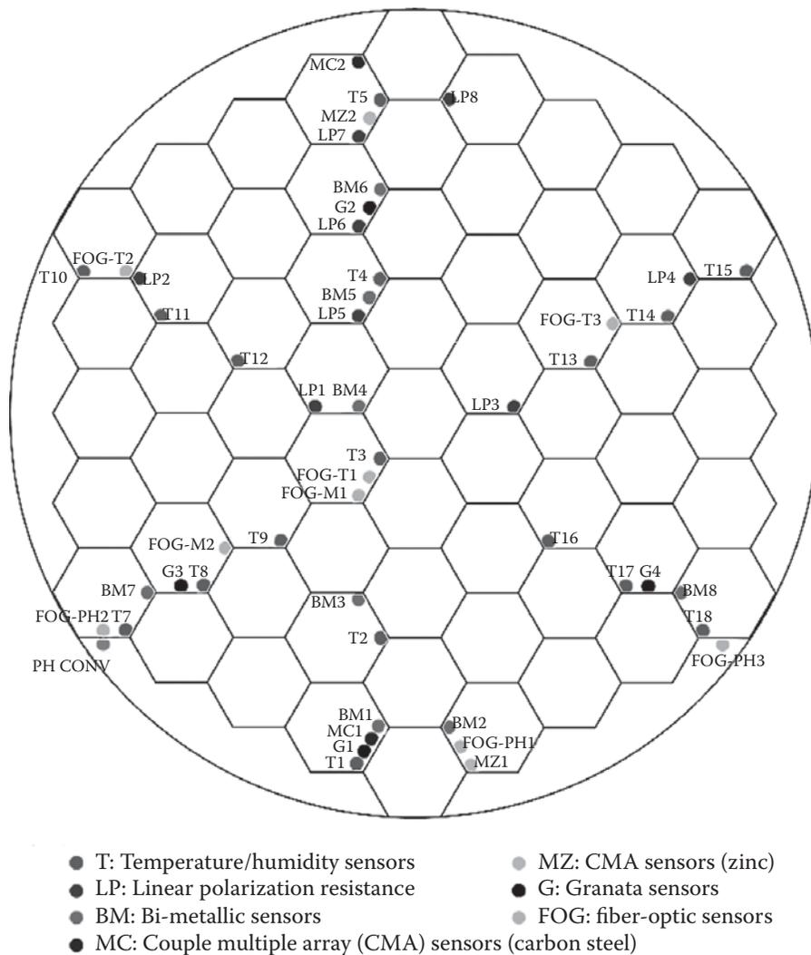
Figure 1.19 Locations of various sensors in the cable model.
