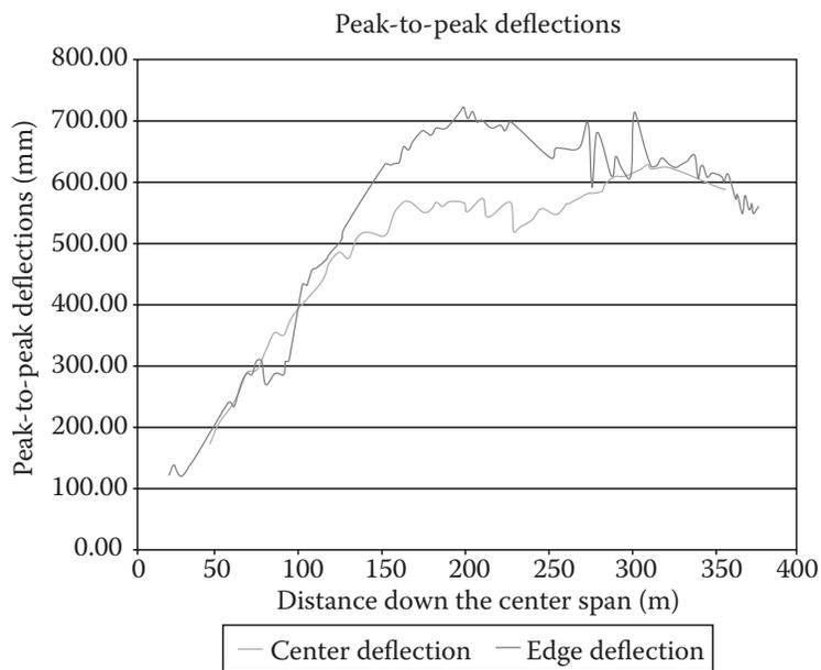
Figure 1.11 Results of interferometric radar scan of half the main span.
