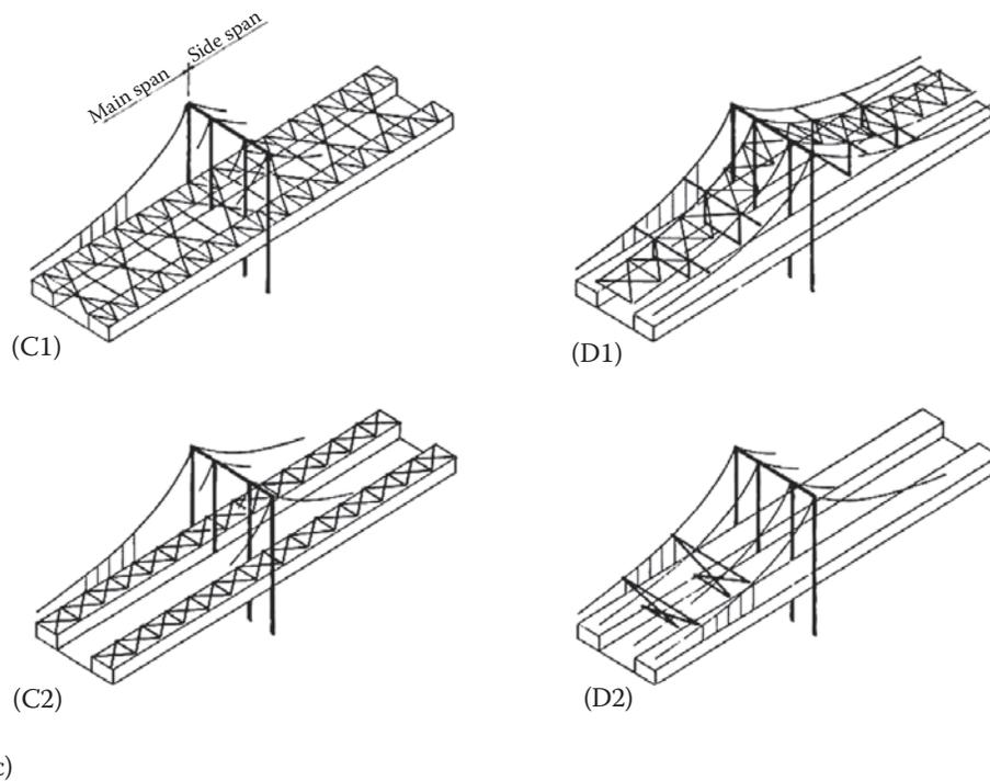
*Figure 1.8 (Continued)* Stiffening schemes. (c) Category C: schemes using torque tubes; (C1) full upper laterals and (C2) partial upper laterals and category D: schemes involving shear on the plane of the cable; (D1) torsional posts and (D2) transverse cables between suspenders.
