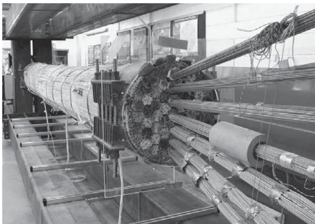
Figure 1.20 Cable model, Carleton Laboratory, Columbia University.
