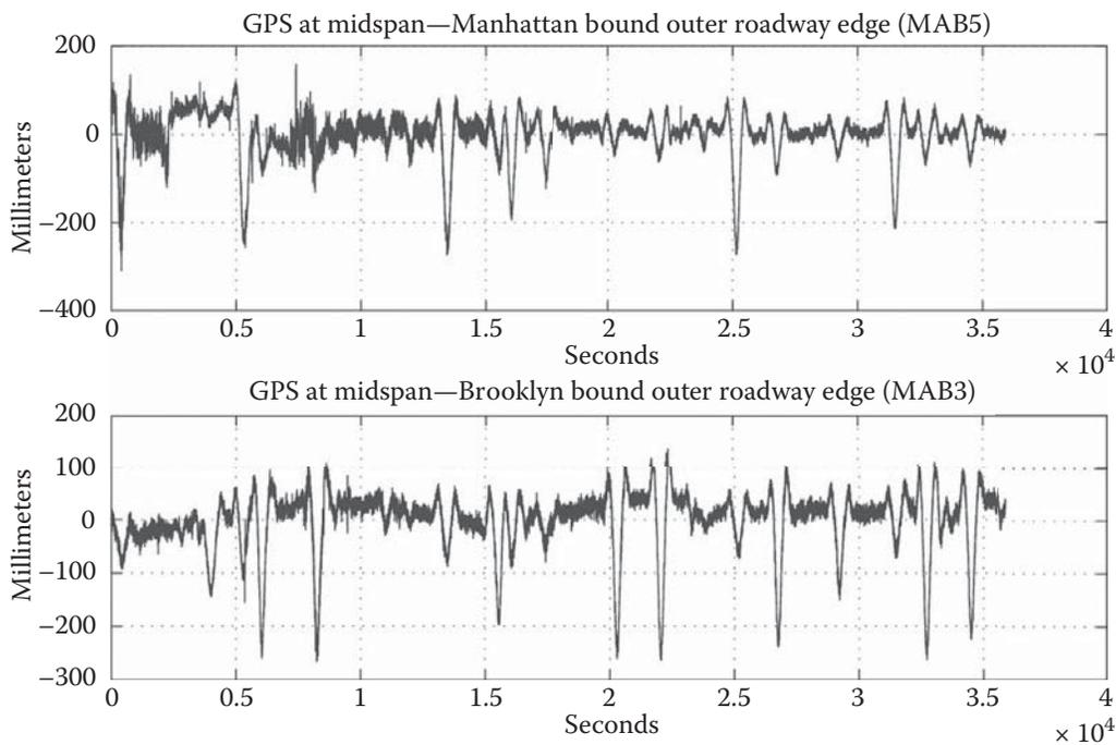
Figure 1.12 GPS receiver data showing outer roadway edge deflections.
