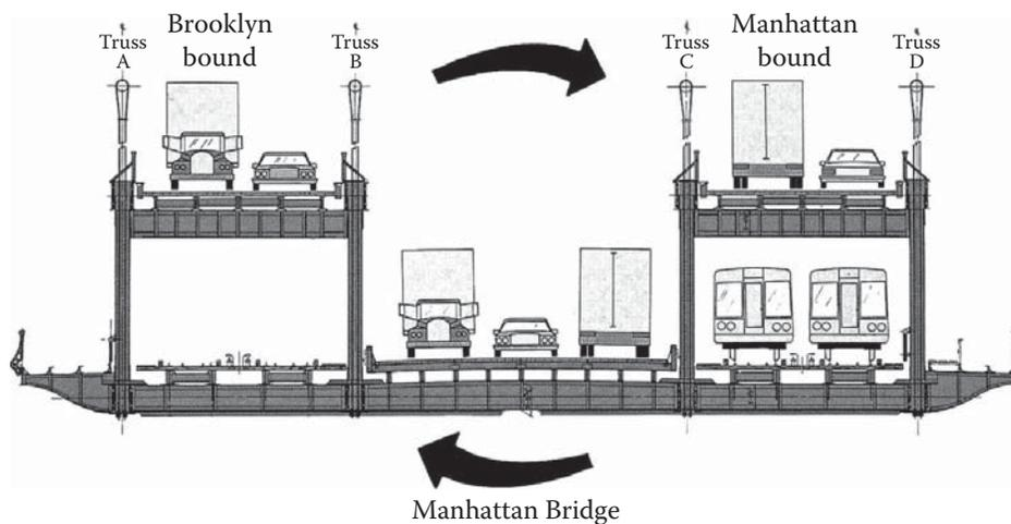
Figure 1.5 Typical cross section with asymmetric loading.
