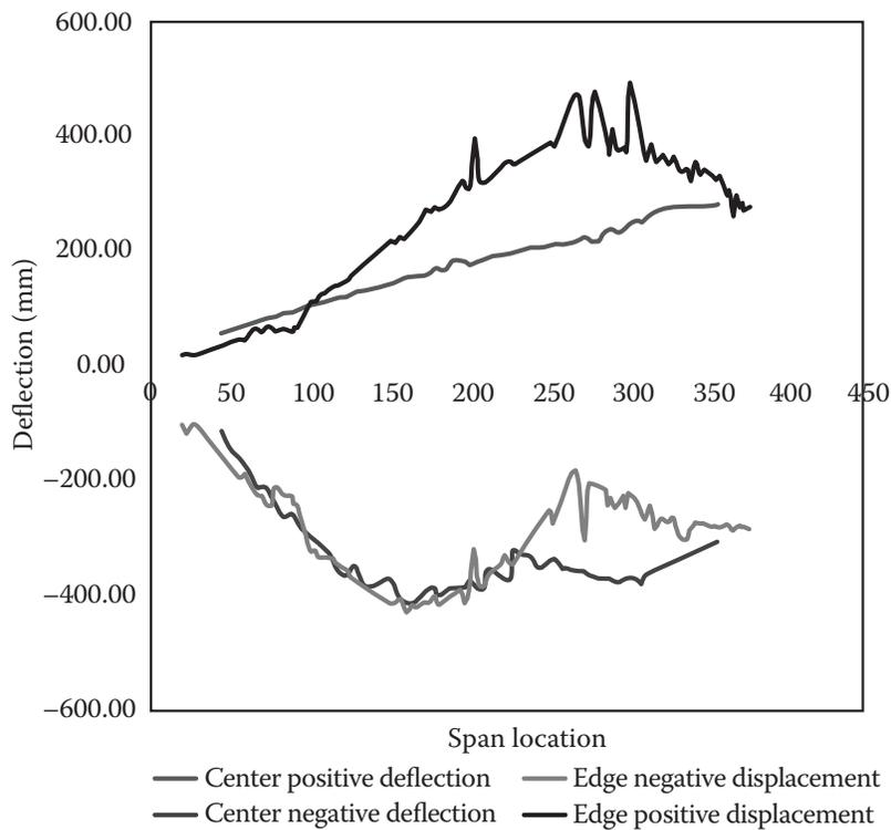
Figure 1.10 Laser tiltmeter measurements of deflection versus span location.
