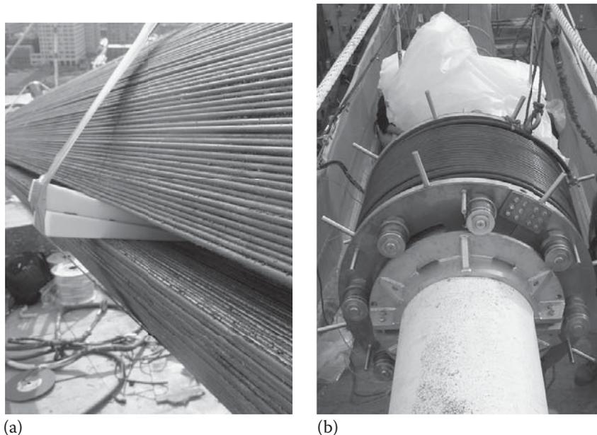
Figure 1.18 (a) Unwrapped wedged cable and (b) testing of cable D by magnetic flux.
