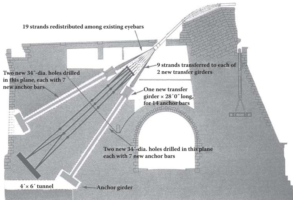
Figure 1.16 Manhattan anchorage, Manhattan Bridge.
