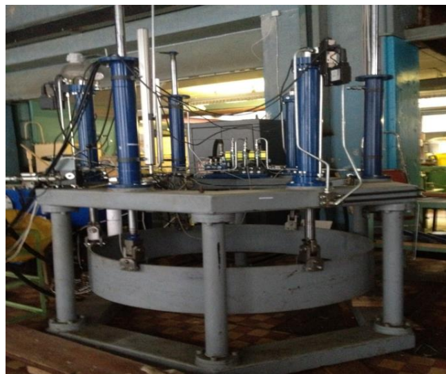
Fig. 7 Testing machine for ring lock
