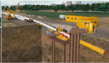
DIRECT PIPE®: One step pipeline installation
